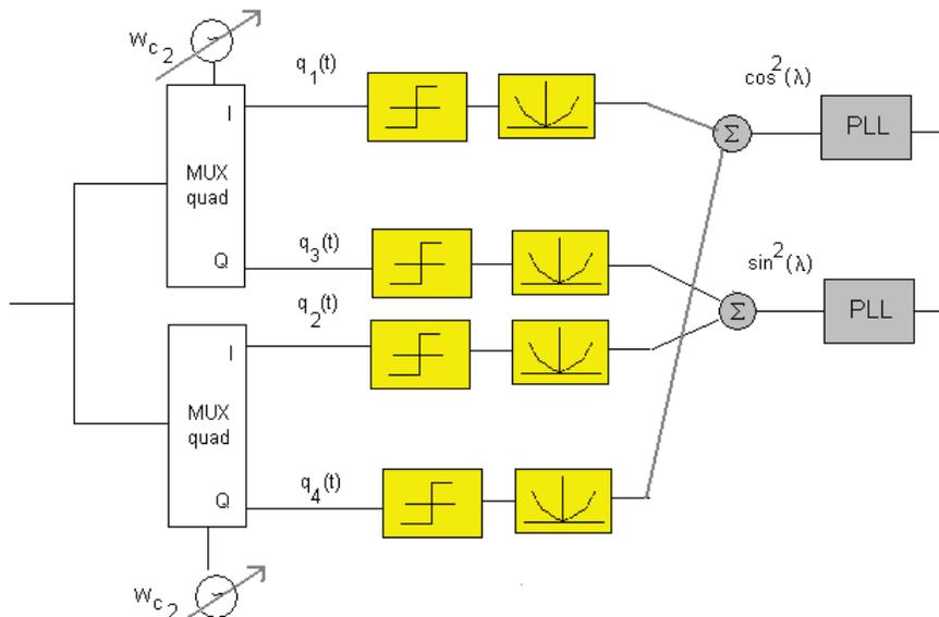
Figure 6. Basic two-carrier Quaternion Demodulator: *In phase* input signal retrieval (Eq.(19c,d)).
