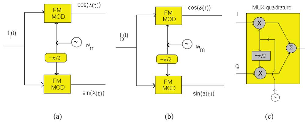
**Figure 3.** Block diagram of circuits for generating quaternion coordinates: a) *in phase* signal drives longitude, b) *in quadrature* signal drives latitude, c) A two-signal basic multiplex used to convey the quaternion coordinates over the same carrier.
