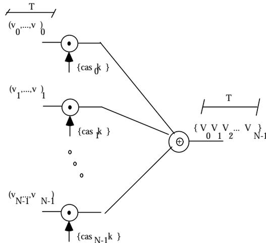
Figure 1. Galois-Field MUX: Spreading sequences.
