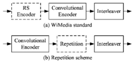
Fig. 4. Possible Coding schemes for the header transmission blocks in WiMedia UWB.
