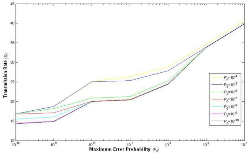
Fig. 2 – Maximum achievable transmission rate as a function of the acceptable error probability.
