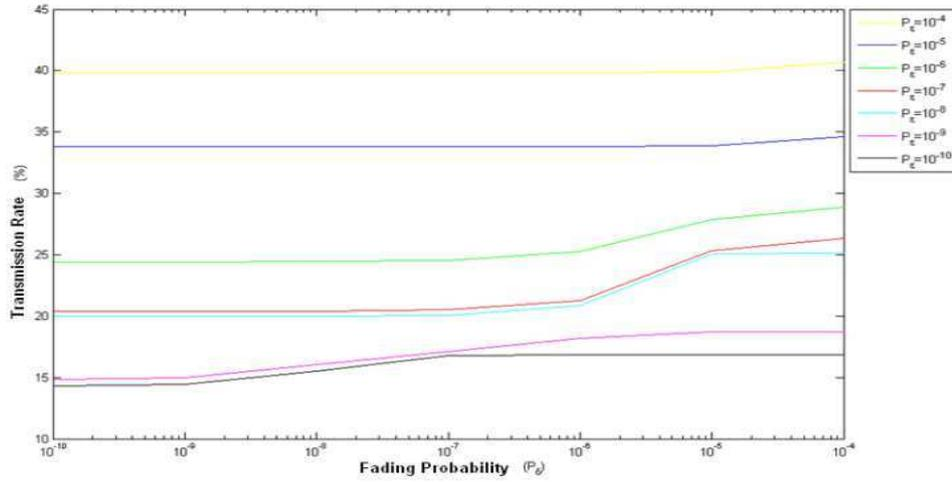
Fig. 1 – Maximum achievable transmission rate as a function of the acceptable erase probability.
