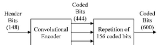
Fig. 5. Convolutional code used in the header of the WiMedia UWB.
