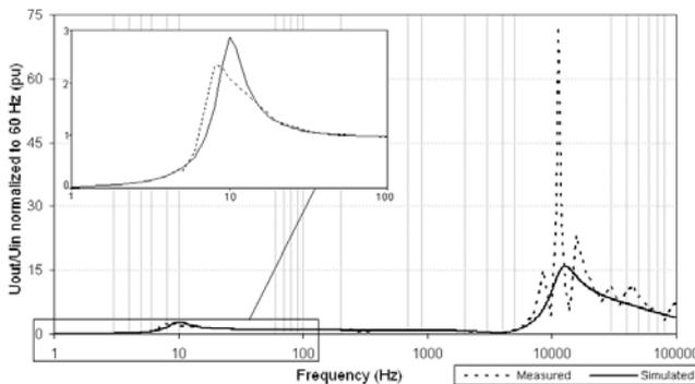
Fig. 6. Simulated and measured frequency response of Type D CCVT.
