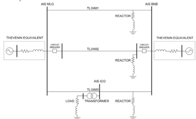
Fig. 7. Transmission system adopted in the digital simulations.
