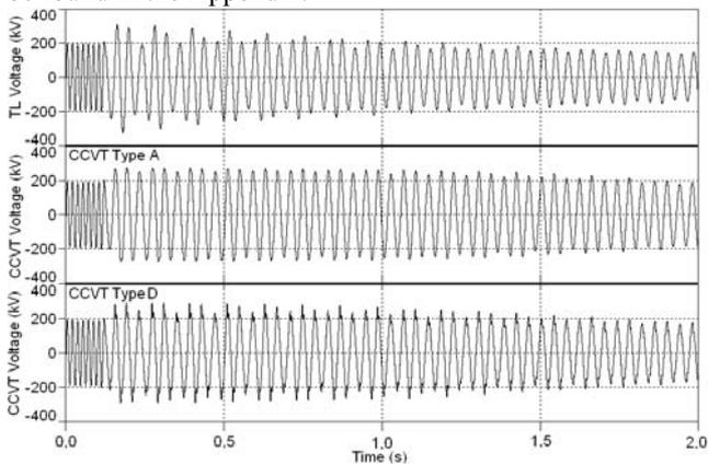
Fig. 12. Performance of Type A and Type D CCVT with  $ZnO$  and rated burden.
