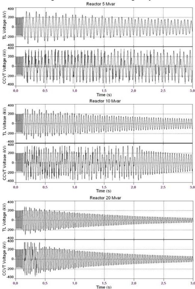
Fig. 8. TL and Type A CCVT Voltages found by ATP simulation.
