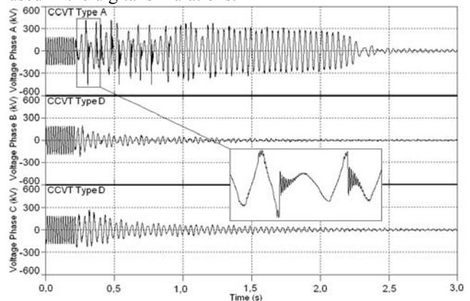
Fig. 13. Oscillographic records of switching-off TL 04M2 (CHESF).
