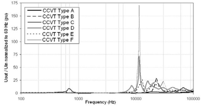
Fig. 4. CCVT Frequency Response (range 100 Hz to 100 kHz).
