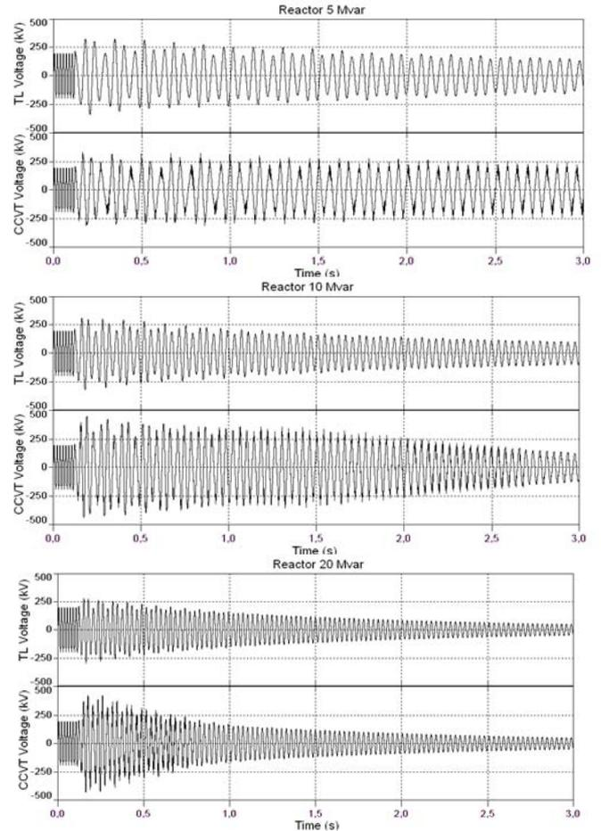
Fig. 9. TL and Type D CCVT Voltages found by ATP simulation.
