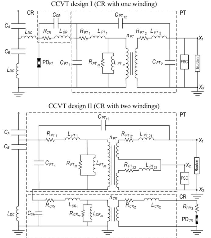
Fig. 1. General CCVT models of two different designs (CR with one and two windings).
