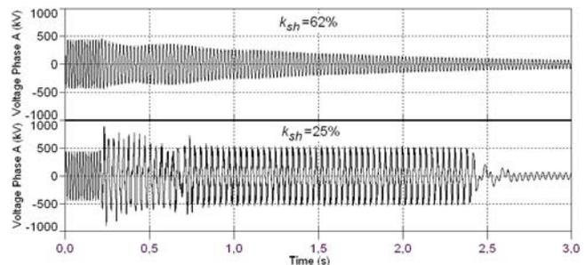
Fig. 14. Oscillographic records of switching-off TL 05C4 (CHESF).
