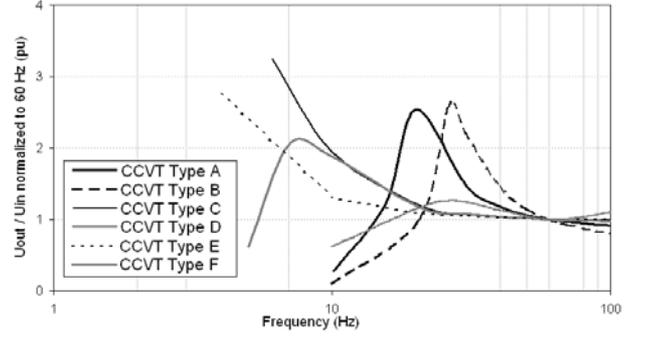
Fig. 3. CCVT Frequency Response (range 1 to 100 Hz).
