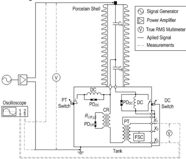
Fig. 2. Frequency response measurements.
