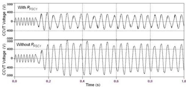
Fig. 11. Performance of Type D CCVT with damage in  $R_{FSC1}$ .
