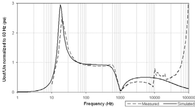
Fig. 5. Simulated and measured frequency response of Type A CCVT.
