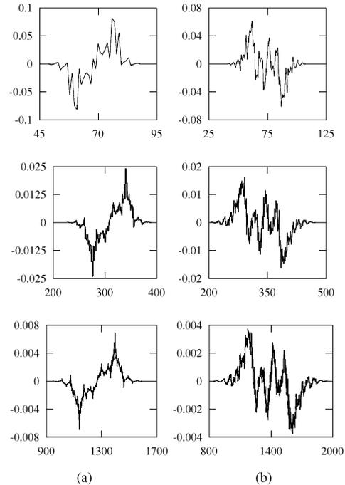
Fig. 2. FIR-based approximation of Mathieu wavelets as the number of iteration increases (two, four, and six iterations, respectively). Filter coefficients holding  $|h| < 10^{-10}$  were thrown away (19 retained coefficients per filter in both cases). (a) Mathieu wavelet with  $\nu = 3$  and  $q = 3$  and (b) Mathieu wavelet with  $\nu = 5$  and  $q = 15$ .
