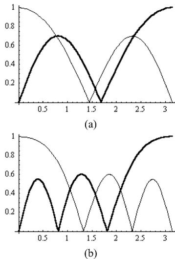
Fig. 1. Magnitude of the transfer function for Mathieu multiresolution analysis filters. (Solid line) Smoothing filter  $|H_\nu(\omega)|$  and (bold line) detail filter  $|G_\nu(\omega)|$  for a few Mathieu parameters. (a)  $\nu = 3$ ,  $q = 3$ ,  $a = 9.915\ 506\ 290\ 452\ 134$ . (b)  $\nu = 5$ ,  $q = 15$ ,  $a = 31.957\ 821\ 252\ 172\ 874$ .
