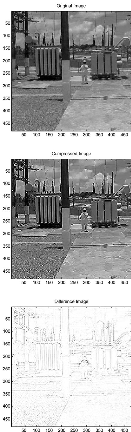
Fig. 8. Image from a 69/13.8kV substation area, its compressed image after two decomposition levels using Geg5ar filter banks and the difference image between them.
